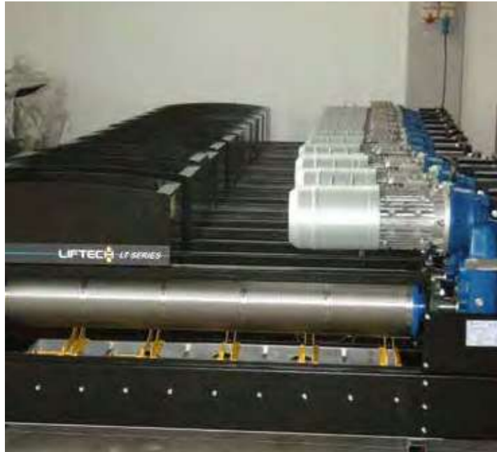
Stage hoists with variable speed Liftech model (Load 500 Kg.)
