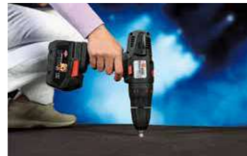
Control of vertical movement by means of a standard electric or battery screwer, introduced into a small central hole in the floor.
